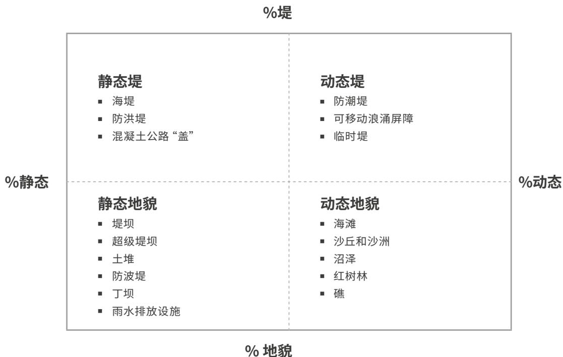
改编自：沿海基础设施：下个世纪适应海平面上升的类型划分(Coastal infrastructure: a typology for the next century of adaptation to sea-level rise)。 (Hill 2015)
